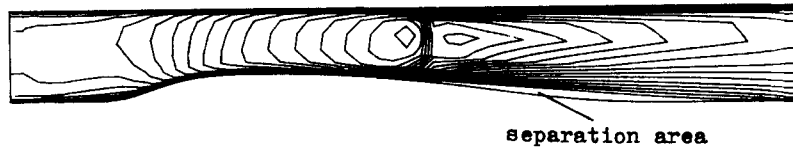
Figure 17. Mach number contours of the calculated viscous flow field for the inlet-diffuser
